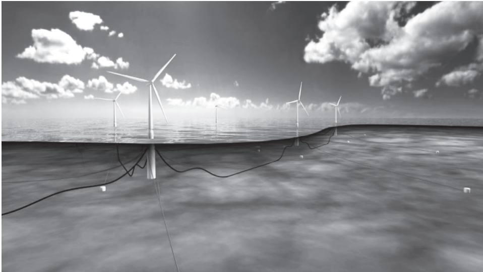
Figure 1.2 Illustration of the Hywind Scotland 30-MW floating wind farm scheduled to be in operation by late 2017 about 25 km offshore from Peterhead. The turbines are each rated 6 MW and the water depth is 95–120 m (Statoil, 2015). Source: Reproduced with permission of Statoil.
