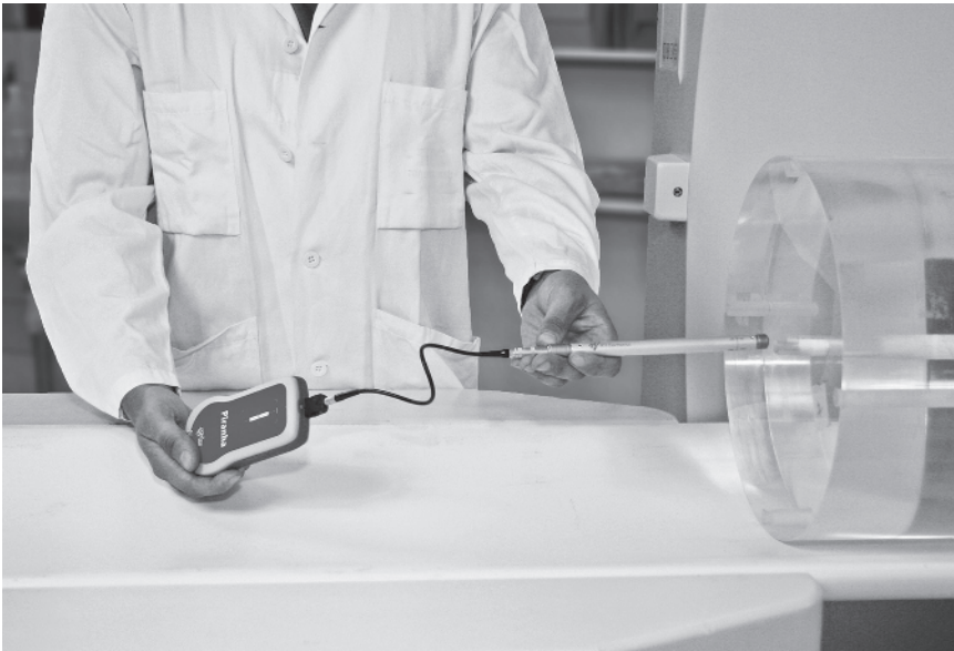
Figure 1.1 Estimating radiation doses from radiological procedures (e.g. CT) by imaging a phantom model of a region of the body with a dosimeter to measure radiation exposure. Source: From info@rtigroup.com.
