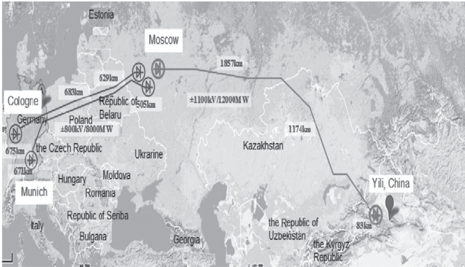
Figure 1.38 Schematic diagram of the Europe, Asia, and Africa intercontinental UHVDC Asynchronous grid interconnection vision. Picture source: SGCC.
