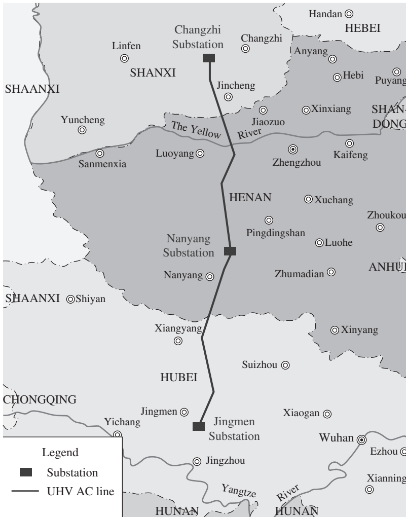
Figure 1.17 Shanxi-Nanyang-Jingmen 1000 kV UHV AC transmission line. Picture source: SGCC.
