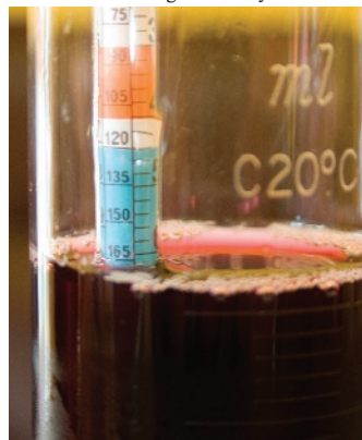
Hydrometer used for measuring sugar content in crushed grapes before fermentation.
