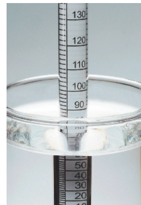
Hydrometer used for measuring alcohol content in a distilled wine sample after fermentation.
