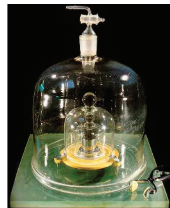
FIGURE 1.14 The international standard kilogram. The pre-2019 SI standard for mass is made of a platinum-iridium alloy and is protected under two bell jars, as shown, at the International Bureau of Weights and Measures in France.
