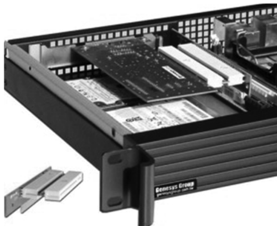
FIGURE 1.21 Riser card in rack server
