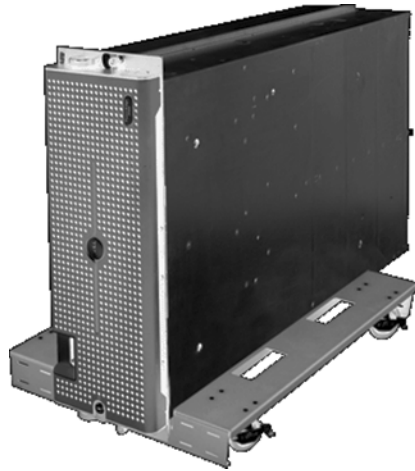
FIGURE 1.6 Tower server in a rack
