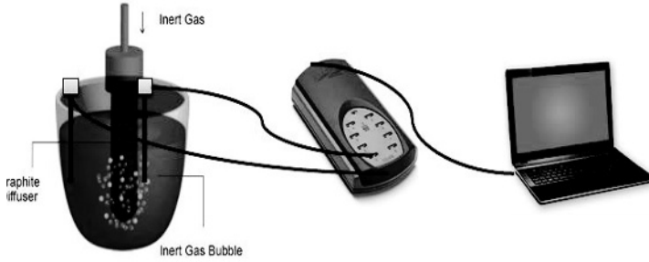
Figure1. Schematic for thermal analysis experiment set-up
