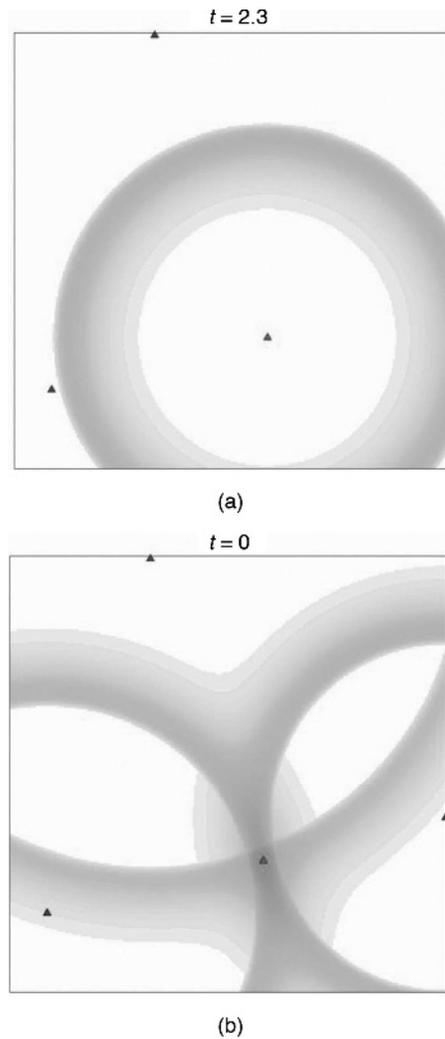
**Figure 1.4** (a) A source emitting an electromagnetic field impulse in free space (triangle at the center of the cylindrical wavefront). Three sensors (triangles on the top, left and right parts of the domain) record the emitted field. (b) Time-reversed waveforms transmitted by the three sensors converge back to the source. (Adapted from [17].) An animated version of this figure can be found on [www.wiley.com/go/rachidi55](http://www.wiley.com/go/rachidi55).
