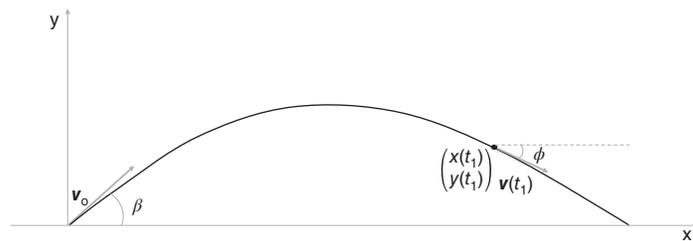
**Figure 1.1** Projectile launched at an angle over a flat earth. The speed and position at time  $t_1$  after the launch are shown after the highest point in the trajectory.
