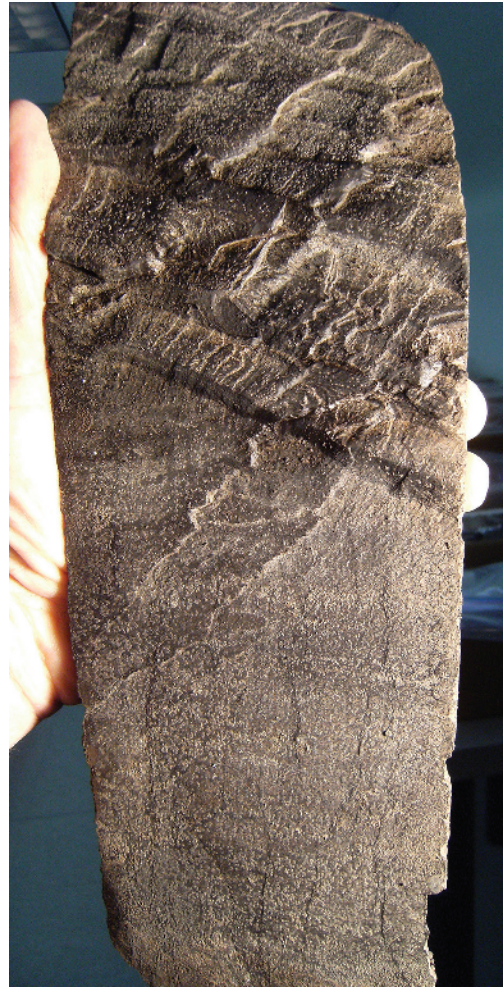
Figure A1b2.3 A fracture plane in a siltstone, without an obvious plume, twisting in the upper half of the core into hackles where the homogeneous rock changes to bedded rock. The twist hackles suggest different mechanical properties and slightly oblique stress regimes in the two zones. Vertical four-inch diameter core, uphole is towards the top of the photo.
