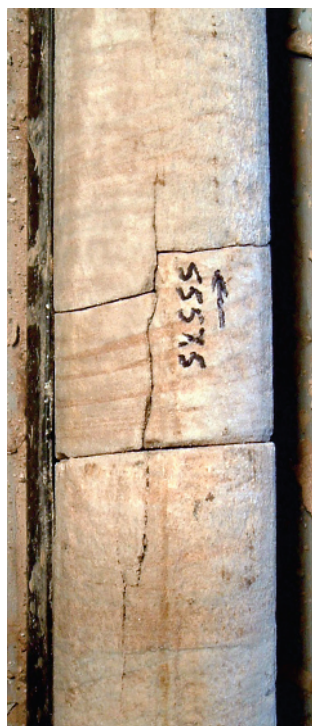
Figure A1c1.10 An irregular high-angle extension fracture that terminates blindly, i.e., for no mechanical reason, in a relatively homogeneous, cross-bedded, anhydrite-cemented, eolian sandstone. Vertical, 2.5-inch diameter core, uphole is towards the top of the photo.
