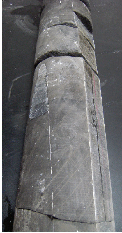
Figure A1e3.1 Two calcite-mineralized vertical extension fractures skim the edge of a limestone core. The fractures intersect at an 80° angle but they have similar characteristics, and the two sets are indistinguishable where they do not occur together in this unoriented core. The importance of recognizing the presence of one versus two fracture sets is that two sets form an interconnected permeability network whereas a single extension fracture set forms a poorly connected network with highly anisotropic drainage and permeability. Vertical 4.5-inch diameter core; uphole is towards the top of the photo.
