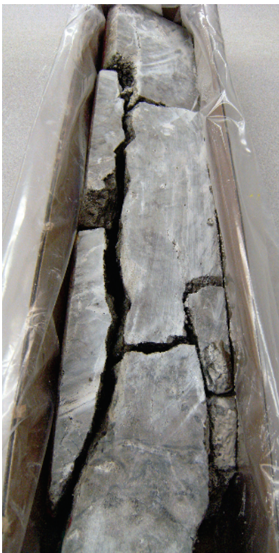
Figure A1d2.2 An irregularly planar extension fracture in a dolomite. If the fracture is irregular in only one plane, i.e., if horizontal cross-sections across this core were to show linear sections of the fracture at any given depth despite this irregularity in the vertical plane shown here, it would be plausibly interpreted as a strike-slip shear fracture, especially if the surface was marked by shear indicators. However, the fracture is likely to be an extension fracture if the fracture surface is irregular in cross-sections oriented in any direction. This core has broken open along the poorly mineralized fracture plane. Butts of vertical four-inch core; up-section is towards the top of the photo.
