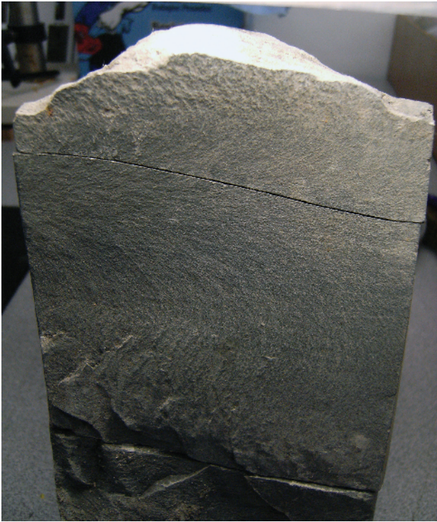
Figure A1d1.1 The plume structure commonly associated with extension fracturing can be formed in many lithologies, including limestone as shown here. Plume structure may be inhibited in coarse-grained lithologies such as conglomerates and crystalline dolomites, but can form easily in these strata if the grains do not offer significant mechanical contrasts or if the stress differential was high enough to drive fractures indiscriminately across the grain boundaries. Vertical, four-inch diameter core; uphole is towards the top of the photo.
