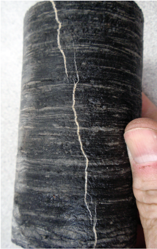
Figure A1d5.2 A calcite-mineralized fracture cuts irregularly through a thinly laminated silt-shale lithology. Poor planarity is a function of lithologic heterogeneity probably combined with a low stress differential during fracturing. Vertical, two-inch diameter core; uphole is towards the top of the photo.
