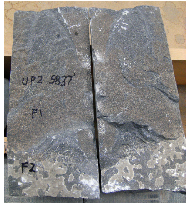
Figure A1e1.6 Intersecting high-angle extension fractures (“NF”) as exposed on the end and slab face of a vertical core. The larger fracture has an irregular width and aperture, suggesting dissolution and indicating good potential for fluid flow. Dissolution-enhanced fractures in this core are oriented at a characteristic angle to the narrower fractures, and the two sets can be distinguished even where they do not intersect. The two planes of exposure, on the slab surface and on the end of the core, illustrate the difference between the true and apparent widths of the larger fracture. Slab from a vertical four-inch diameter core; uphole is towards the top of the photo.
