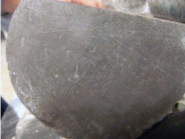
Figure A1d4.3 Two sets of narrow, intersecting, calcite-mineralized, high-angle extension fractures exposed on the end of a core cut from a calcareous shale. The single fracture cutting upper right to lower left predates the other fractures since they terminate against it. Examination of the slab face alone, or even of the slab in three dimensions, would not have revealed the second fracture set; the second fracture set is apparent only in the butt section of the core. Butts of a vertical, four-inch diameter core; uphole is towards the viewer.
