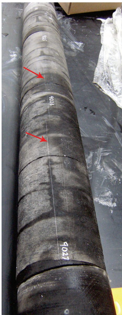
Figure A1c1.3 Two overlapping, narrow, calcite-mineralized, high-angle extension fractures with dips parallel to the core axis so that the full heights can be measured and logged. Vertical four-inch sandstone core, uphole is towards the top of the photo.
