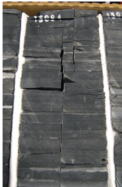
Figure A1c1.16 Some overlapping en echelon offsets occur at mechanical discontinuities such as variations in lithology. Here, the propagation of a fracture in shale was inhibited by thin limestone beds, but equal strain across the formation created a new fracture that propagated in a parallel, offset plane. Slabs of vertical, four-inch core, uphole is towards the top of the photo.
