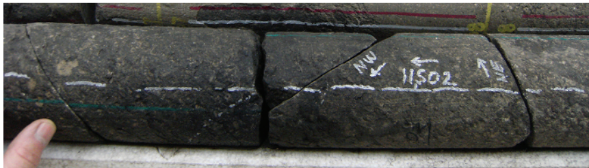
Figure A1e3.2 Fracture planes in horizontal cores can also be extended beyond the core volume to projected intersections. Here two sets of high-angle extension fractures in a horizontal core have strikes that intersect at nearly 90°, but the intersections are not captured within the core. The silver line marks the high or dorsal side of the core. A quick, conceptual image of the reservoir fracture system, consisting of a network of closely spaced, high-angle fractures with 90° intersections, can be developed from this core. Horizontal three-inch diameter core; uphole is to the left of the photograph.
