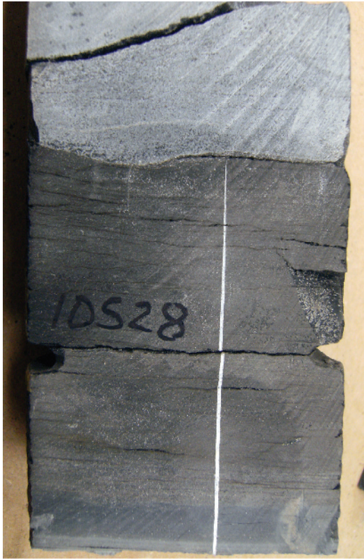
Figure A1c1.5 Mechanical properties can change over geologic time due to diagenesis and changes in pore pressures. Some clay-rich lithologies that are presently relatively ductile were, under different conditions, the more fracture-prone strata in a heterogeneous sequence. In this example, a calcite-mineralized vertical extension fracture in a shale tapers towards its termination against a limestone layer. At the time of fracturing, the shale was more susceptible to fracturing than the limestone. Slab from a vertical three-inch diameter core, uphole is towards the top of the photo.
