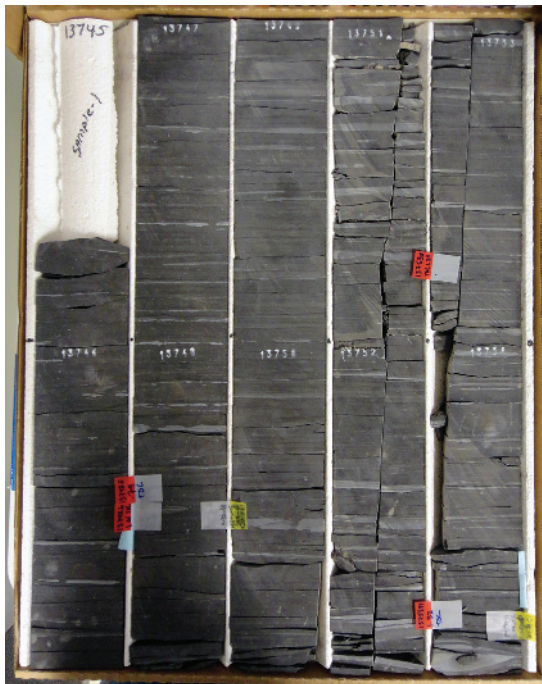
Figure A1c3.4 Two views of closely spaced, strata-bound, parallel, unmineralized, high-angle extension fractures. Left: fractures are parallel to the white lines, and are confined to thin siliceous shale beds bounded by thinner clayey shale beds. Right: same piece of core, looking from the top down and showing the two closely spaced fractures in the upper layer of siliceous shale. The presence of this many fractures suggests that despite the small sample size, the core captured a representative population of both spacings and heights, and that the reservoir is intensely fractured. Vertical 3.5-inch core; uphole is towards the top of the photo (left) and towards the viewer (right).
