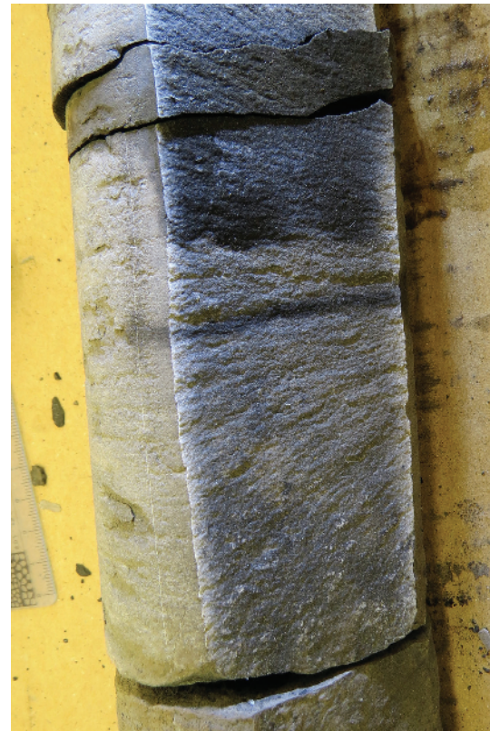
Figure A1b1.3 A large-scale plume records the propagation of this fracture face from right to left across the core, which was cut from a non-calcareous shale. The plume is without a well-defined axis but propagated upward and to the left in the upper half of the cored fracture, and downward and to the left in the lower half. The fracture is lightly mineralized with calcite but the plume relief is greater than the thickness of the layer of calcite and the ornamentation is apparent through the mineralization. Vertical four-inch diameter core, uphole is towards the top of the photo.
