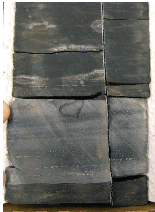
Figure A1d3.8 A relatively wide (2 mm), incompletely mineralized, near-vertical extension fracture that extends indiscriminately across shale and limestone beds. The fracture surfaces are slightly rougher in the limestone but otherwise there is little difference in fracture characteristics in the two lithologies. Mineralization consists of two layers of calcite attached to the fracture faces and growing inward, with euhedral crystal faces marking a medial, unmineralized aperture. Slabs of vertical, 3.5-inch diameter core; uphole is towards the top of the photo.
