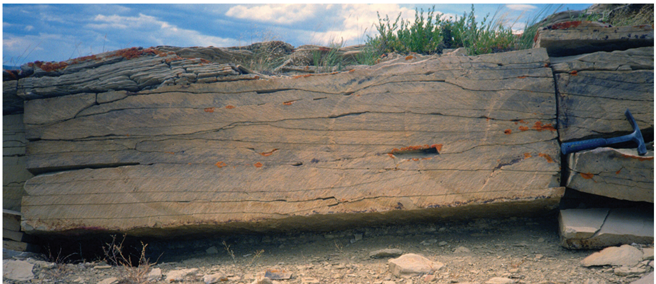
Figure A1b.3 Extension fracture in a sandstone showing an origin near the end of the hammer handle, possibly at the cross fracture, and an initial circular shape where the fracture radius was less than the thickness of the host bed. The fracture subsequently propagated incrementally, both left and right, pausing long enough in several places to create arcuate arrest lines. The plume pattern is normal to the arrest lines.
