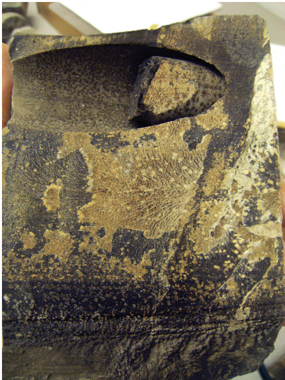
Figure A1b1.5 A subtle plume propagated horizontally from right to left across this fracture face. The strata-bound fracture, in a non-calcareous siltstone, is covered by a layer of diagenetic clay half a millimeter thick. The impression of the plume from the missing half of the fracture is preserved on the surface of the clay. Vertical four-inch diameter core, uphole is towards the top of the photo. The stump of an unsuccessfully recovered one-inch diameter porosity/permeability plug remains in the hole cut into the core.
