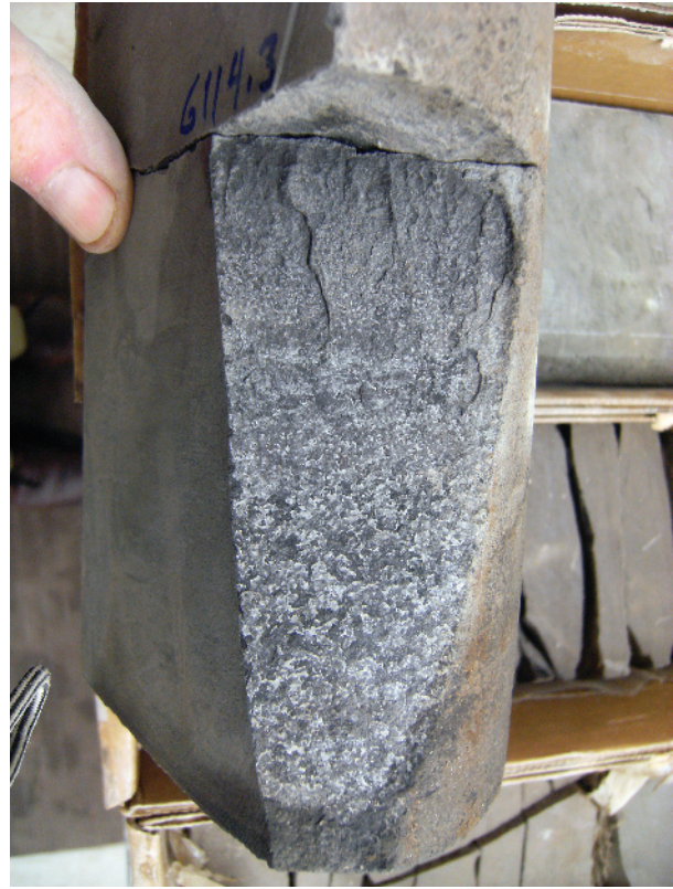
Figure A1c1.6 A near-vertical, calcite-mineralized fracture exits the core downward before reaching its termination, and terminates upward, with twist hackle, against a lithologic boundary. The upward decrease in the thickness of the calcite mineralization corresponds to a narrowing of the fracture. Vertical four-inch diameter limestone core, uphole is towards the top of the photo.
