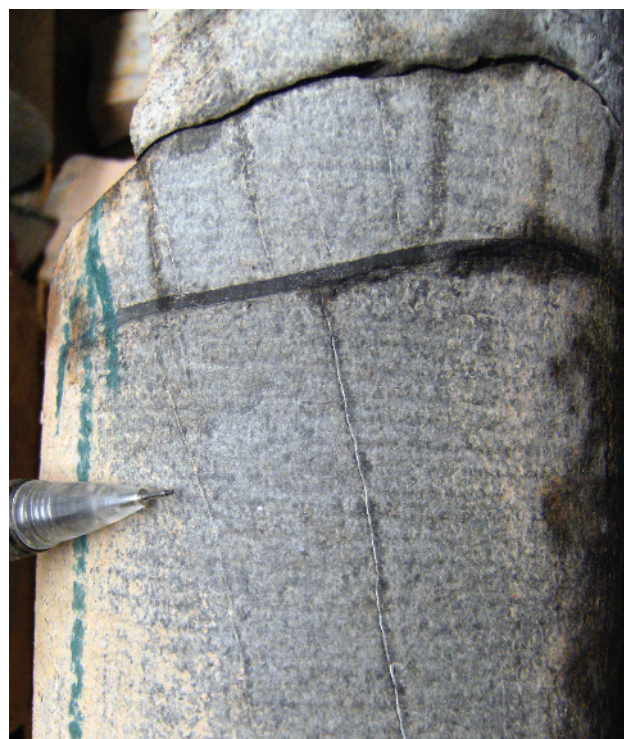
Figure A1c1.4 Even thin shale layers can provide enough mechanical contrast to arrest the propagation of extension fractures, suggesting that the energy required to form this type of fracture is relatively low. Vertical four-inch diameter limestone core, uphole is towards the top of the photo.
