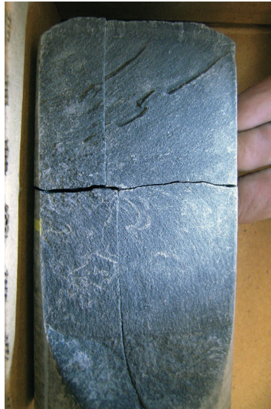
Figure A1b1.7 A plume with a horizontal axis, highlighted by oblique lighting, records the propagation of an extension fracture from left to right in a fine-grained limestone interbedded in a shale sequence. The top edge of the fracture is marked by minor twist hackle where it approaches a shale layer. The bottom edge of the natural fracture terminates at another bedding plane but without twisting. The fracture plane was extended downward along the rougher curved surface during core processing, exiting the core towards the viewer. The vertical line in the fracture face is the slabbing saw cut. Vertical three-inch diameter core, uphole is towards the top of the photo.
