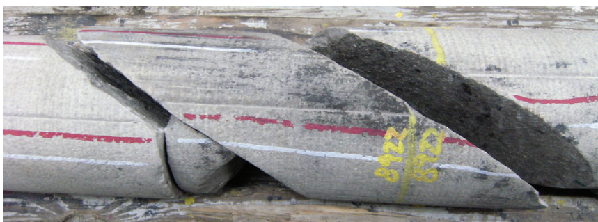
Figure A1c3.7 The spacings of high-angle extension fractures can be measured directly in many horizontal cores. The scribe-line groove next to the red line on the core surface indicates that this sandstone core was mechanically oriented relative to stratigraphic up, and the fractures were determined to be vertical, corroborated by their orientation normal to bedding. Bedding planes may be horizontal, but there can still be a 180° ambiguity as to top vs. bottom of the bedding. That ambiguity was resolved for this core with the orientation survey. Fracture spacing normal to the fracture planes, as opposed to their spacings along the core axis, can be measured directly. Note that the “uphole” core orientation line pair has non-standard colors: red is on the right looking uphole as usual, but a white line replaces the more common black line in the pair. In horizontal cores, “uphole” refers to the direction towards the heel of the well and then upward to the surface. Two red–white line pairs were marked on this core so that both the slabs and butts would be marked after slabbing, but there can be confusion if the pairs are drawn too close together. Horizontal four-inch diameter core; uphole is to the left.
