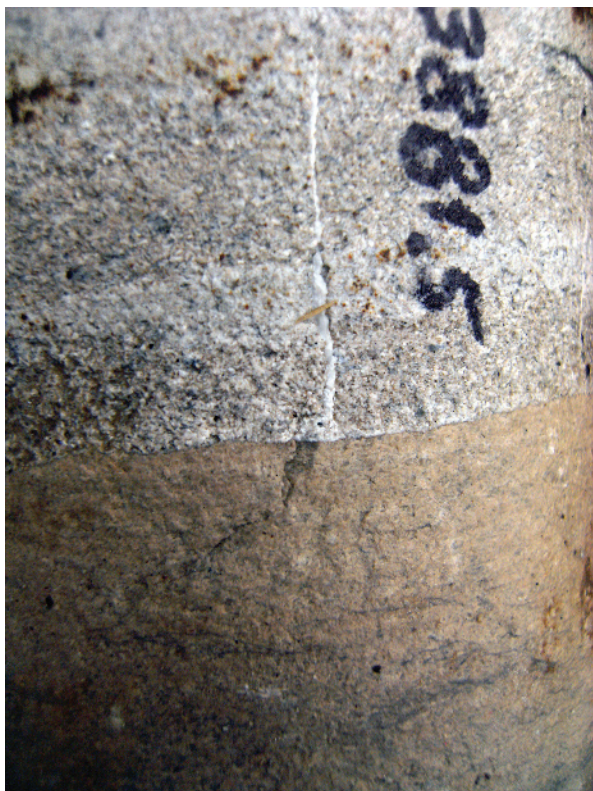
Figure A1c1.8 A strata-bound, calcite-cemented vertical extension fracture in a gray dolomite terminates abruptly, without tapering, at a contact with an adjacent limestone. Vertical four-inch diameter core, uphole is towards the top of the photo.
