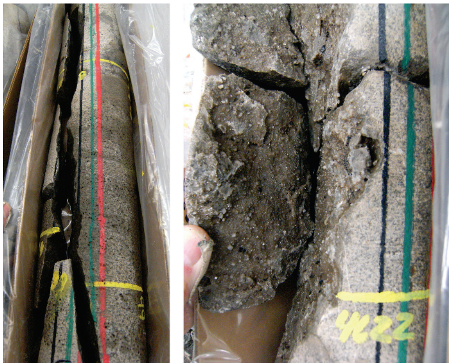
Figure A1d2.3 Left: a tall high-angle extension fracture in a coarsely crystalline dolomite has a rough, irregular plane. The core has broken open along the incompletely mineralized fracture plane. The green line between the red–black uphole/downhole orientation lines is a Master Orientation Line useful for assessing fracture strikes relative to each other in continuous intervals of core. Right: scattered millimeter-scale dolomite crystals are present on the faces of a fracture from the same formation and fracture system. Some of the irregularity of this fracture is due to postfracturing dissolution. The dolomite crystals were precipitated after dissolution. Vertical four-inch diameter core: uphole is towards the top of both photos.
