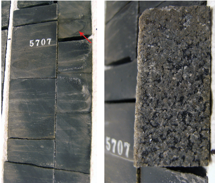
Figure A1d3.2 Two views of a tall high-angle extension fracture in shale. The fracture is approximately 3 mm wide. The photo on the right shows the face of the fracture on the piece of core indicated by the arrow in the photo on the left. In contrast to the fracture shown in the previous photo, both fracture faces are incompletely mineralized with calcite that grew from the walls into the open aperture. Irregular mineralization indicates that this fracture creates an important conduit to fluid flow, with permeability significantly greater than that of the matrix of the host rock. Slabs of vertical, four-inch diameter core; uphole is towards the top of the photo.
