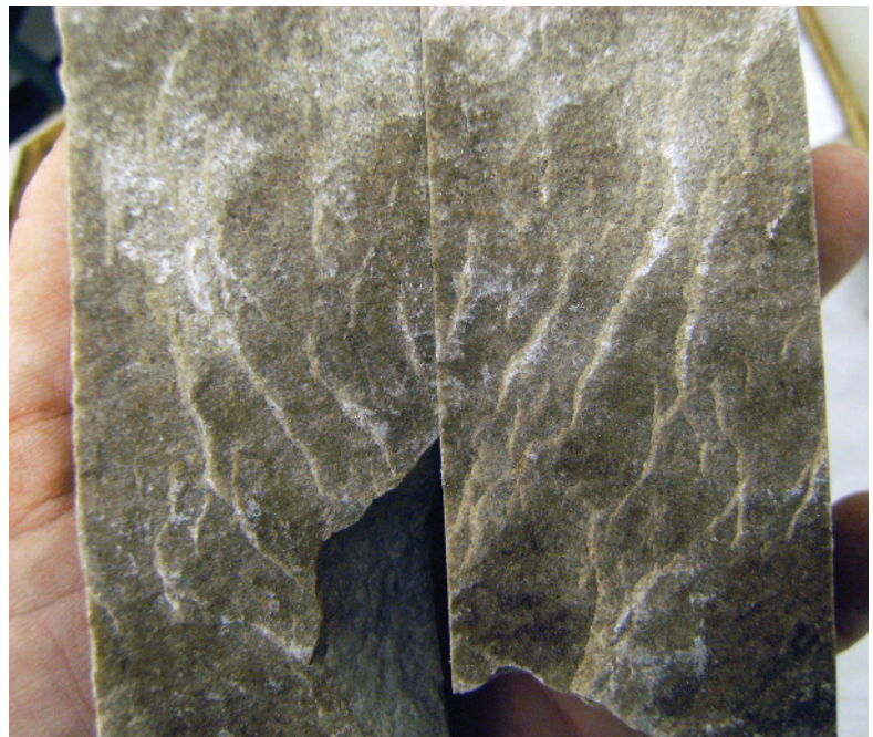
Figure A1b2.4 Opposing faces of a vertical extension fracture in oil-stained sandstone that show twist hackle transitioning upward into a more planar extension fracture. The fracture face is not marked by plume structure since the sandstone is poorly cemented and not mechanically prone to the formation of plumes. Vertical three-inch diameter core, uphole is towards the top of the photo.
