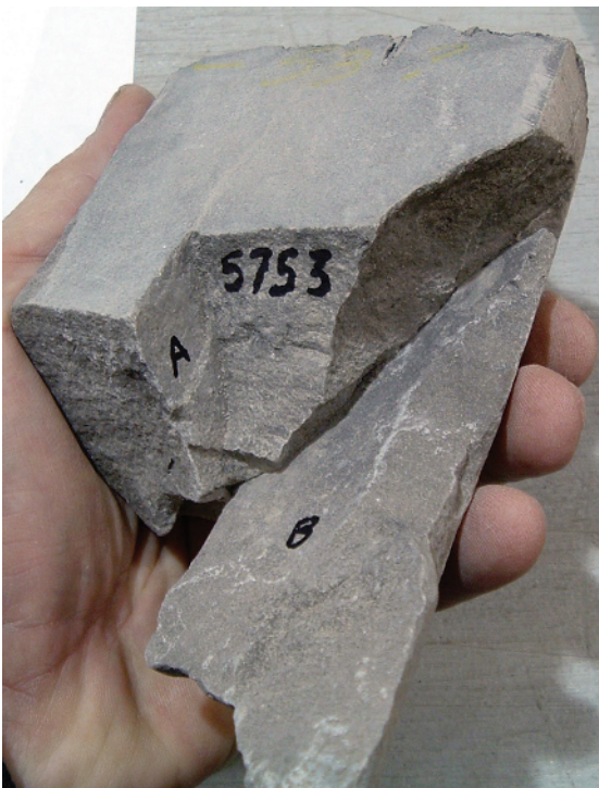
Figure A1e2.1 Fragments of two high-angle extension fractures (planes marked A and B) in the butts of a core cut from dolomite. Only one of the fractures intersects the slab plane. Vertical three-inch diameter core; uphole is towards the top of the photo and away from the viewer.
