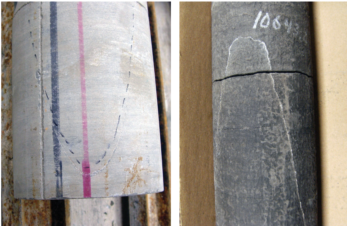
Figure A1c1.12 Full fracture height cannot be measured where the fracture exits the core top or bottom before terminating. In the example on the left, the location and type of termination at the base of a calcite-mineralized extension fracture are unknown since the fracture exits the side of the core downward (the fracture is highlighted by the dashed line marked on the core surface beside the fracture trace). In the right photo it is the upper termination that is unknown. Even though truncated, minimum heights can and should be measured. Vertical, four-inch diameter limestone (left) and shale (right) cores; uphole is toward the tops of both photos. The core on the left was also oriented relative to north, as indicated by the scribe groove immediately to the left of the black line. The red–black line pair in this photo is the most common convention for marking the in situ up orientation of a core, with “red on the right looking uphole.”
