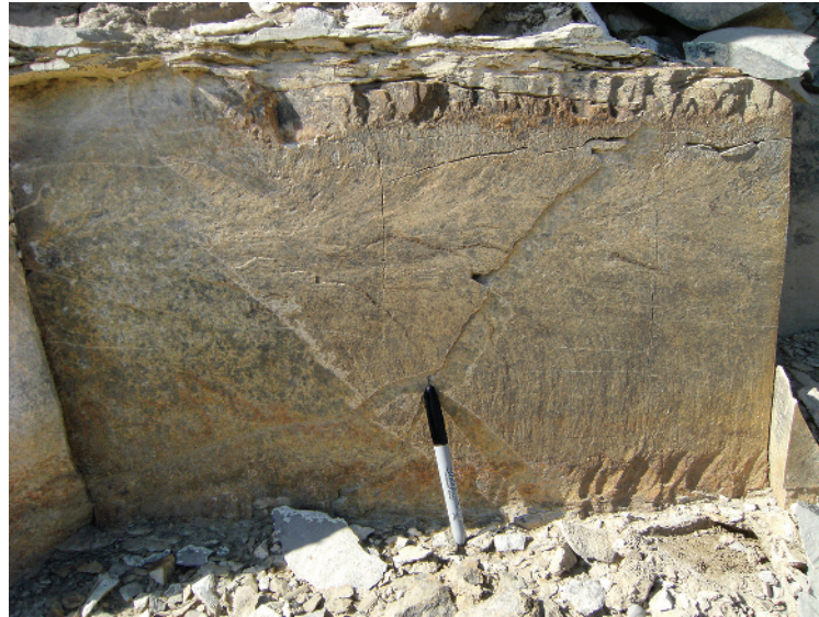
Figure A1b.2 A strata-bound fracture decorated with a faint plume structure that propagated from left to right, and that broke into twist hackle in the altered stress areas near the upper and lower bedding contacts.
