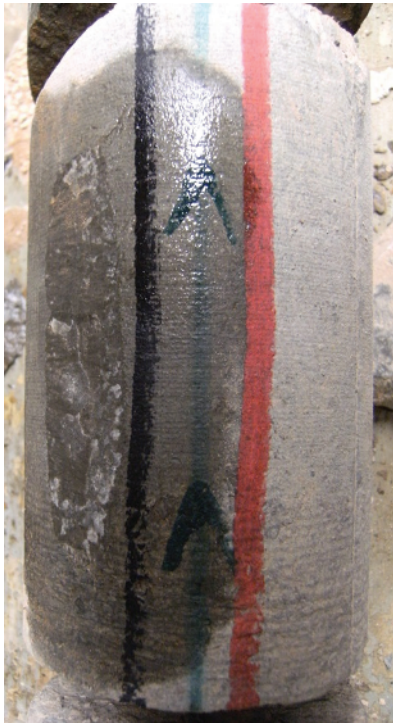
Figure A1c1.13 One face of a high-angle extension fracture skims the edge of this core. A small but important data set can be recorded from this example, including parameters such as the presence of fracturing, a minimum fracture height and width, and the fact that the fracture is mineralized with calcite but that the mineralization is weaker than the host rock. Fracture strike might also be addressed if this fracture plane can be related to the strike of other induced or natural fractures. Vertical, four-inch diameter limestone core; uphole, as marked by both the red-black line pair and the uphole arrows, is towards the top of the photo.
