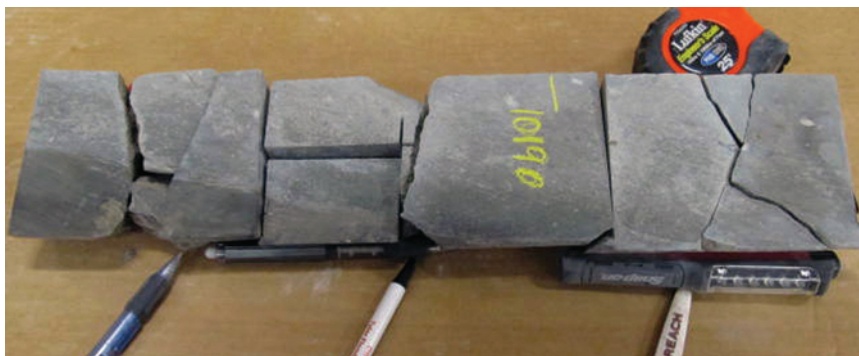
Figure A1c3.6 High-angle extension fractures in a near-horizontal core, in a glauconitic limestone near the contact with an underlying shale. Three parallel natural fractures are located at the tips of the blue pencil, the white pen, and the white toothbrush handle (the toothbrush is used for cleaning the core). The flashlight and gray pencil lying parallel to the core were used for stabilizing the core pieces for the photograph. The bed-normal natural fractures are obscured by various saw cuts and induced breaks in the core. If this spacing were typical of the reservoir, a vertical core would have about a 75% chance of capturing one of these three fractures. However, fractures are more widely spaced, of the order of 10 ft, in the middle of the limestone, reducing the probability of fracture intersection to about 3%. Butts of four-inch core; uphole is towards the right of the photo.
