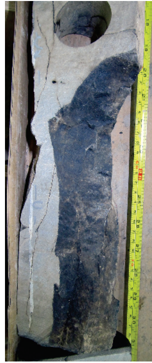
Figure A1d5.4 High-angle extension fractures can also be irregular in structurally complex settings. This oil-stained extension fracture in a limestone is from a faulted anticline. Complex fractures such as this may be related to local structural complications. Vertical, four-inch diameter core; uphole is towards the top of the photo.
