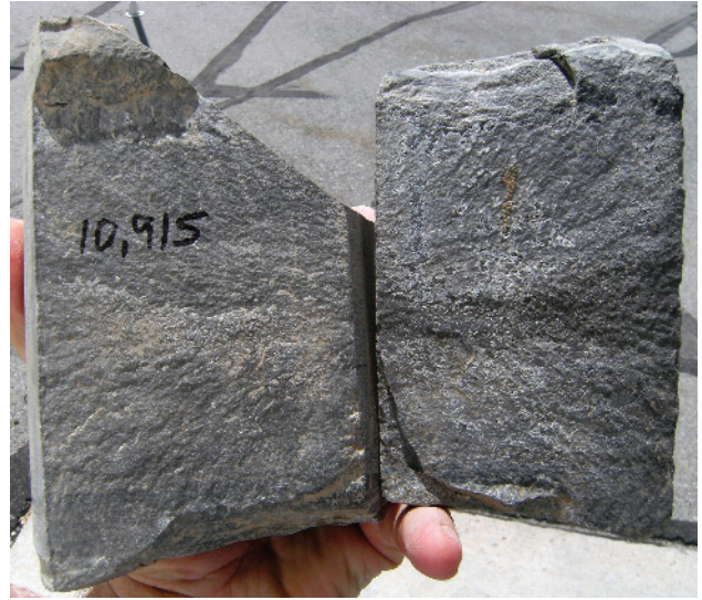
Figure A1b1.6 Opposing faces of an extension fracture in limestone show mirror images of the plume structure on the two surfaces. The fracture grew horizontally in this rock. The narrow fracture is lightly mineralized with calcite on both faces. Vertical four-inch diameter core, uphole is towards the top of the photo.
