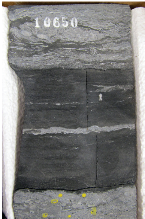
Figure A1d3.6 Two incompletely mineralized, high-angle extension fractures that are confined to shale units interbedded with shell-hash limestones. At the time of fracturing, the shale was more susceptible to brittle deformation than the limestone. Slabs of vertical, four-inch diameter core; uphole is towards the top of the photo.
