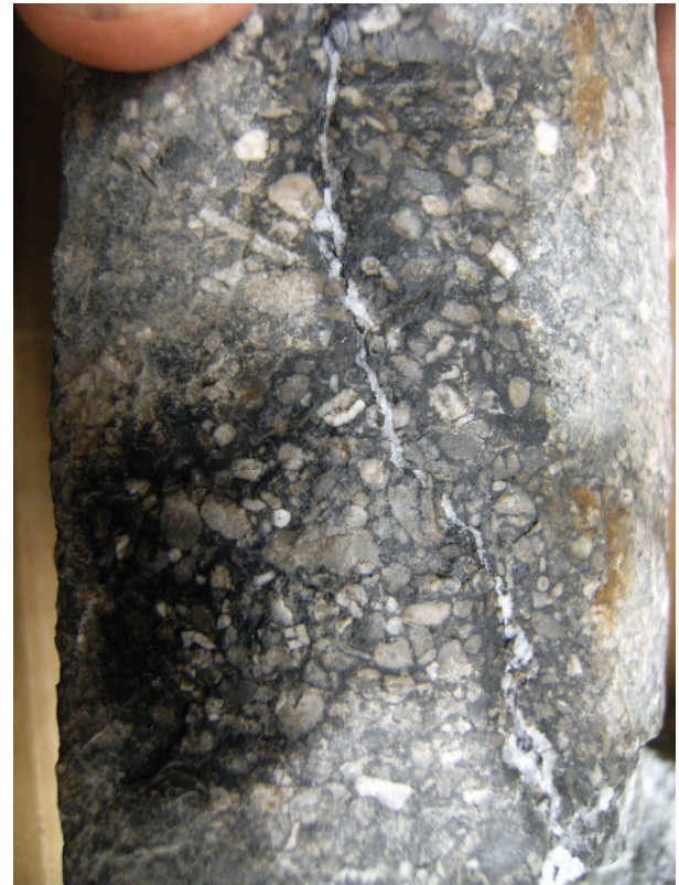
Figure A1d5.1 Some extension fractures found in coarse-grained rock such as in this bioclastic limestone are irregular, the fracture planes having propagated around rather than through the clasts. Vertical three-inch diameter core; uphole is to the top of the photo.
