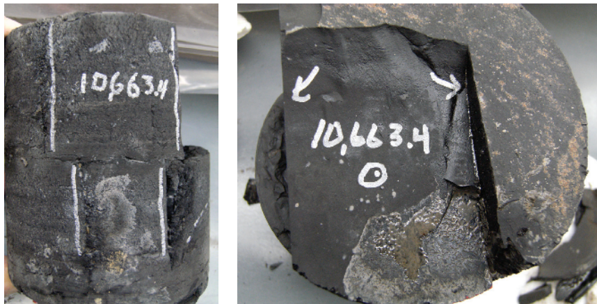
Figure A1c3.4 Two views of closely spaced, strata-bound, parallel, unmineralized, high-angle extension fractures. Left: fractures are parallel to the white lines, and are confined to thin siliceous shale beds bounded by thinner clayey shale beds. Right: same piece of core, looking from the top down and showing the two closely spaced fractures in the upper layer of siliceous shale. The presence of this many fractures suggests that despite the small sample size, the core captured a representative population of both spacings and heights, and that the reservoir is intensely fractured. Vertical 3.5-inch core; uphole is towards the top of the photo (left) and towards the viewer (right).
