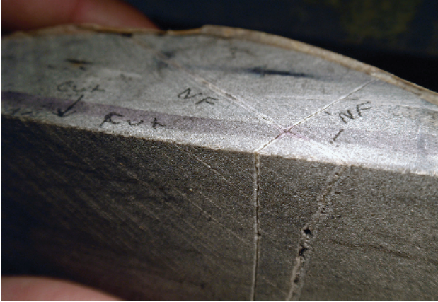
Figure A1e1.6 Intersecting high-angle extension fractures (“NF”) as exposed on the end and slab face of a vertical core. The larger fracture has an irregular width and aperture, suggesting dissolution and indicating good potential for fluid flow. Dissolution-enhanced fractures in this core are oriented at a characteristic angle to the narrower fractures, and the two sets can be distinguished even where they do not intersect. The two planes of exposure, on the slab surface and on the end of the core, illustrate the difference between the true and apparent widths of the larger fracture. Slab from a vertical four-inch diameter core; uphole is towards the top of the photo.
