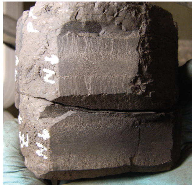
Figure A1b2.2 Two short, parallel, laterally offset, strata-bound extension fractures in a strongly bedded siliceous shale. A subtle plume structure marks the lower fracture but none is evident on the upper fracture. The upper fracture, however, is marked by well-developed, low-relief twist hackle along both the upper and lower edges. Vertical three-inch diameter core, uphole is towards the top of the photo.
