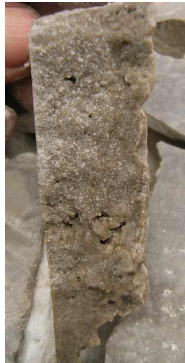
Figure A1d1.3 Two views of a rough-surfaced, high-angle extension fracture (between the two arrows in the left photo) in a vuggy, coarse-grained limestone. The photo on the right shows the fracture face, with subtle crystalline calcite mineralization. Plume structure is unlikely to have developed on such irregular fractures in coarse-grained lithologies, but plumes are also easily removed by dissolution in soluble lithologies. Slab of a four-inch, vertical core; uphole is towards the top of both photos.
