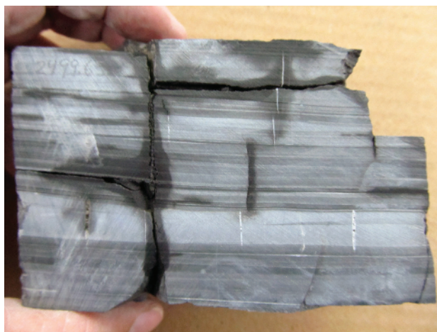
Figure A1c1.7 Short, calcite-mineralized, strata-bound fractures that are confined to brittle limestone layers and that terminate abruptly against the interbedded ductile shales. Slab from a vertical four-inch diameter core, uphole is towards the top of both photos.
