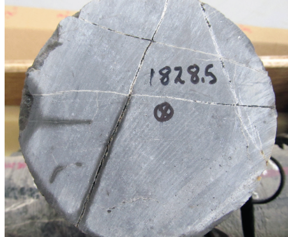
Figure A1e1.5 Four calcite-mineralized but incompletely filled fractures with at least three distinct strikes in core cut from a limestone. The relative ages of the fractures are unclear. Water has wicked into the aperture of the lower left fracture indicating significant remnant fracture porosity. Vertical, four-inch diameter core. The circled X indicates that the view is uphole.
