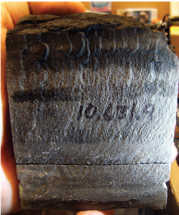
Figure A1b2.1 Definitive twist hackle growing out of a poorly defined left-to-right plume structure, marking the changed mechanical properties and stress conditions near the bedding contact and the upper edge of the fracture. Vertical three-inch diameter core, uphole is towards the top of the photo.
