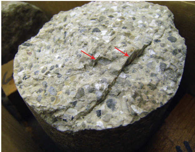
Figure A1d5.3 Extension fractures can be planar even in coarse-grained rock such as this pea-gravel conglomerate, if the rock was well cemented, if the clasts had mechanical properties that are similar to those of the matrix material, and/or if the stress differential that drove fracturing was high. Vertical four-inch diameter core; uphole is towards the viewer.
