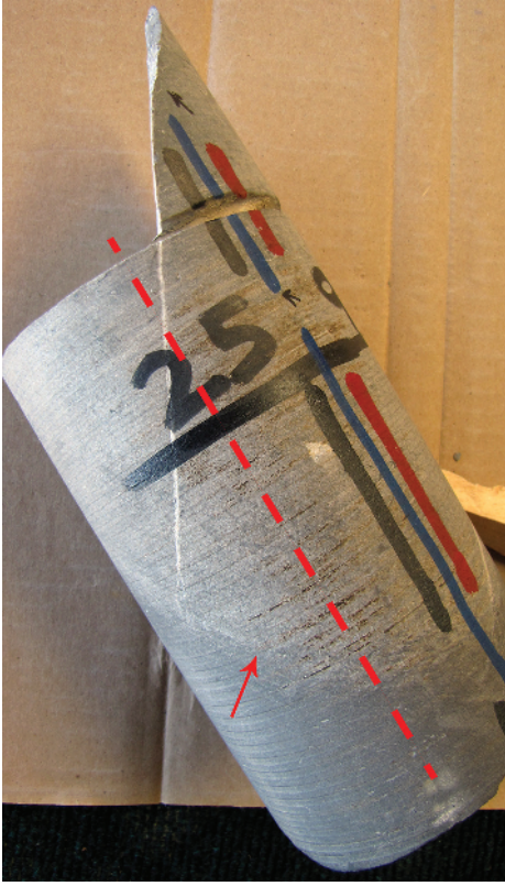
Figure A1f.3 A calcite-mineralized vertical fracture in a piece of unslabbed sandstone core cut from a wellbore that is deviated at about 50^\circ from the vertical. The core has been propped up into its in situ position. There is only one position of rotation around the central core axis (indicated by the red dashed line) at which the bedding (arrow) is horizontal and the fracture is vertical. Fracture strike can then be physically measured using the wellbore deviation azimuth. If bedding is absent or not horizontal, and/or if the fractures are not vertical, the problem becomes more complicated. Deviated, four-inch diameter core; uphole is towards the upper left corner of the photo, stratigraphic up is towards the top of the photo.
