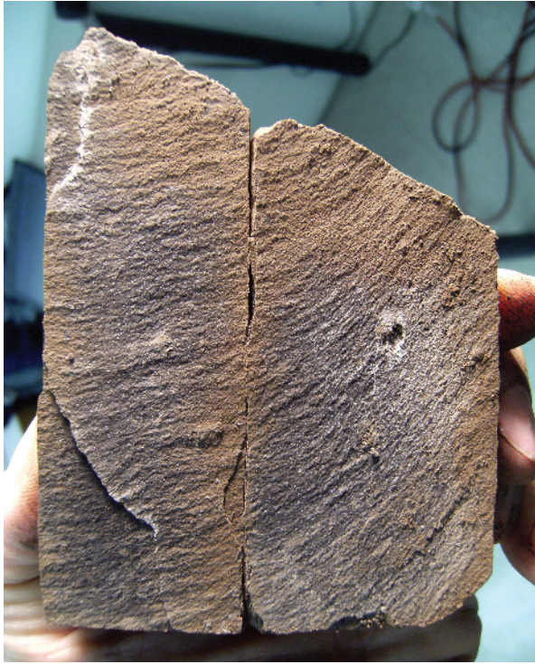
Figure A1b1.4 This core captured part of a plume that was much larger than the core. The fracture is mineralized with a light layer of calcite. Remnants of drilling mud (tan) stain the fracture face. Vertical four-inch diameter core, uphole is towards the top of the photo.
