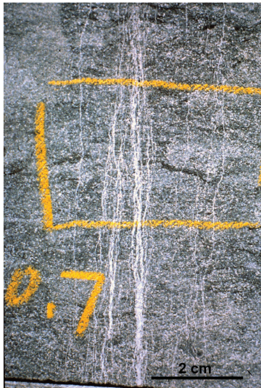
Figure A1d4.4 Bundled, narrow, high-angle extension fractures in a deeply buried sandstone. Thin sections (location marked by the yellow rectangle) show fractures both cutting through grains and following grain margins. Slab face of a vertical four-inch diameter core; uphole is towards the top of the photo.
