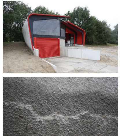
45 Microscopic view of self-repairing concrete. Self-repairing concrete incorporates calcite-precipitating bacteria. The bacteria create minerals that repair cracks in concrete.
