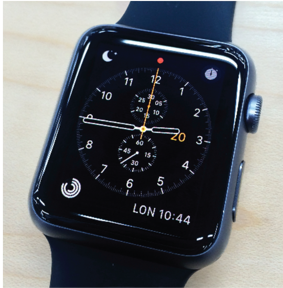
Figure 1.3 Example of a smart watch using active-matrix OLED (AMOLED) (Apple Watch Series 2 by Apple).
