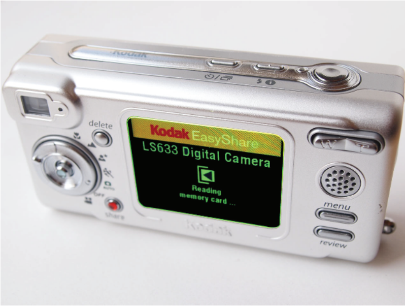
Figure 1.1 The first active-matrix OLED display product on the market (Kodak LS633 digital camera).
