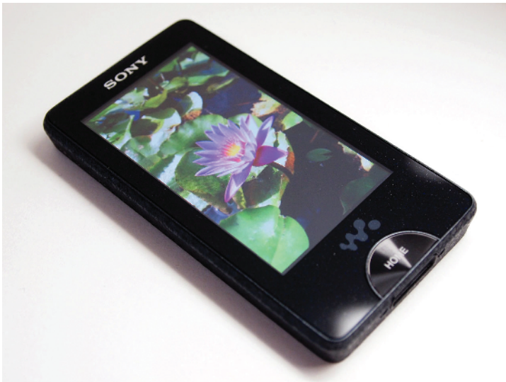
Figure 1.4 Example of an audio player using active-matrix OLED (AMOLED) (Sony Walkman NW-X-1050).
