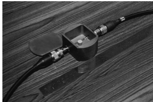
Figure 1.13 The experimental setup for measuring the quality factor by the strip line method. The DR is coupled to the strip line.
