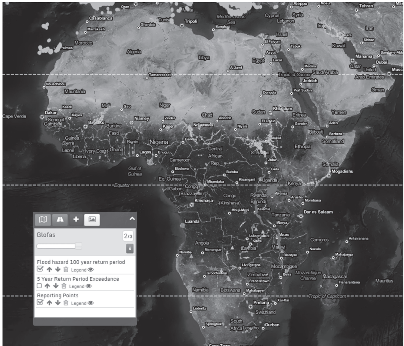
Figure 1.4 Pan-African flood hazard map for the reference return period of 100 years, as displayed on the GloFAS website ( http://globalfloods.jrc.ec.europa.eu/ ).
