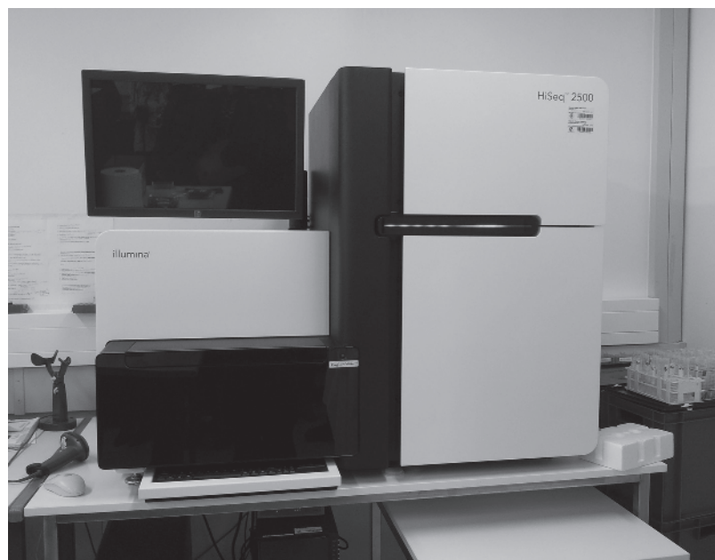
Figure 1.5 A typical optical DNA sequencer.
