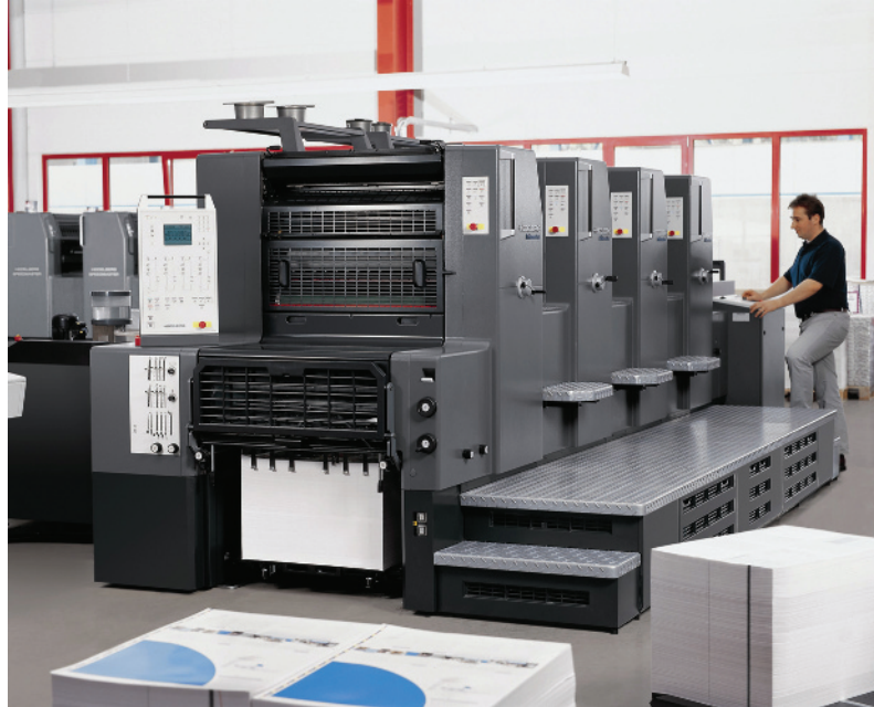
Figure 1.19 A standard profile such as GRACoL or FOGRA51 is used to represent the color characteristics of a printing press such as this 4-color Heidelberg Printmaster 74, sheetfed, offset press. Source: Heidelberg. Reproduced with permission of Heidelberg®.
