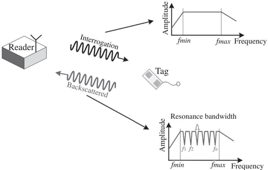
**Figure 1.6** Working basis of the frequency-domain chipless RFID systems.
