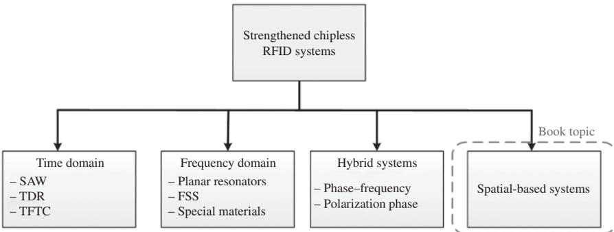
Figure 1.5 General classifications of chipless RFID systems.
