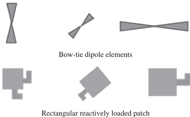
**Figure 1.7** Phase-domain-based chipless RFID tags.
