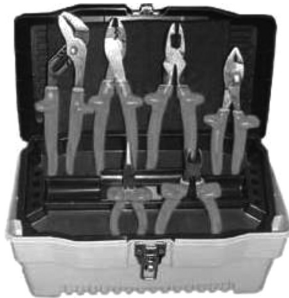
Figure 1.7 Typical insulated tools. Source: Reproduced with permission of OSHA.
