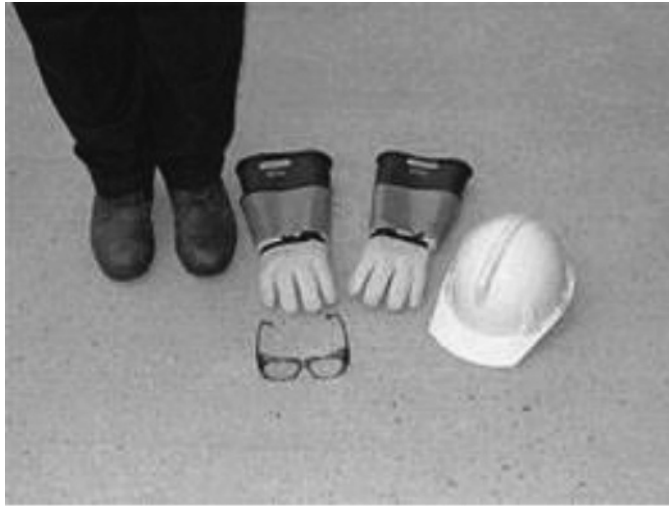
Figure 1.5 Photo of typical shock protection PPE. Source: Reproduced with permission of OSHA.
