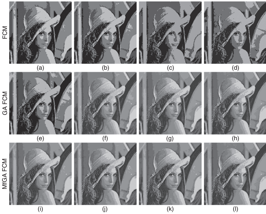
Figure 1.3 8-class segmented 256×256 grayscale Lena image with the class levels obtained by (a–d) FCM, (e–h) GA-based FCM, and (i–l) MfGA-based FCM algorithms of four results of Table 1.2, with Q as the quality measure.
