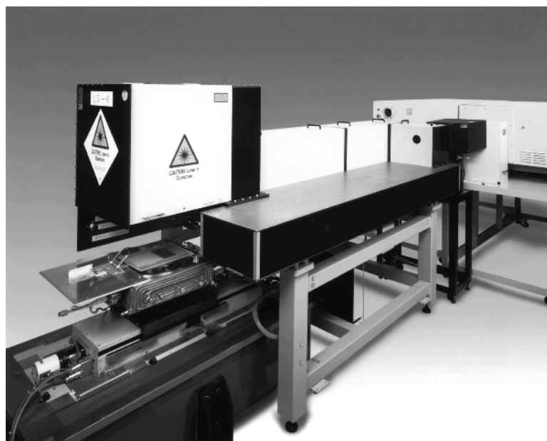
Figure 1.2 Linear-beam laser equipment developed by SEL. Source: Reproduced from [17]. Copyright (2014), with permission from Wiley
