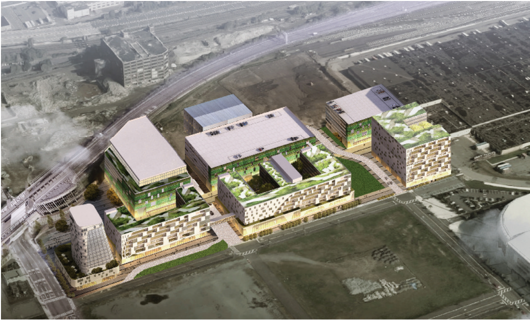
FIGURE 1.6 Harrison Mixed-Use Transit Oriented Development, Harrison, New Jersey. GRO Architects is using BIM in the early design stages of large-scale planning projects. By linking variables like program, assigned by material; number of stories; and metrics for unit and parking count, our practice is exploring way to scale BIM technology to urban plans.
