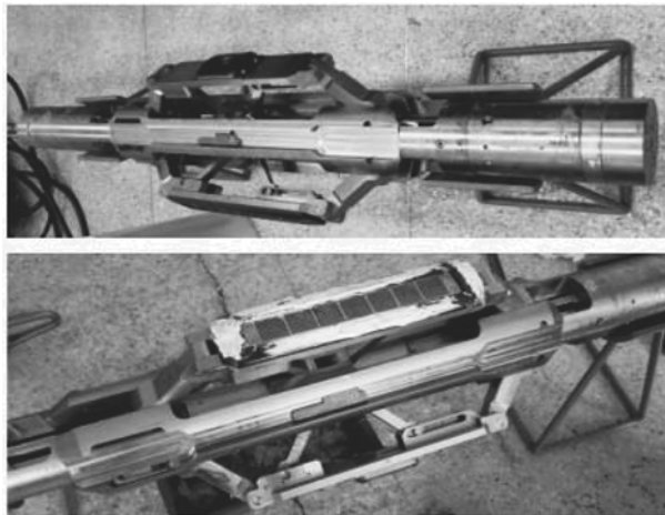
Figure 1.20. New triple probe formation tester. Pads with “small round nozzle and slot probe” (top) and “all long slot nozzles” (bottom).
