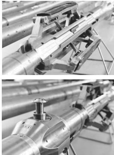
Figure 1.21. New COSL triple probe tester, perspective view.
