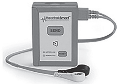
Figure 5.5 Real-time continuous cardiac monitoring system and Heartrak Smart from M/s Mednet Healthcare Technologies, United States.
