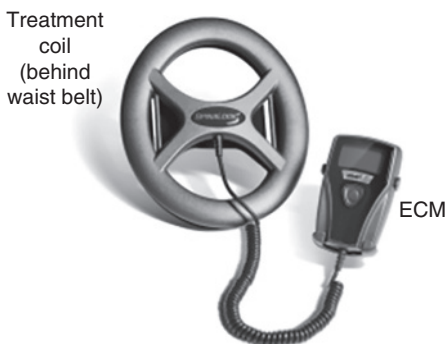
Figure 57.6 SpinaLogic bone growth stimulator. The electronic control module (ECM) and the transducer coil are shown. The module includes a signal generator that produces an electrical signal, which is transmitted to the treatment transducer. The transducer coil is an elliptically shaped copper wire coil that converts the electrical signal into an electromagnetic field. Source: Photograph Courtesy of M/s DJO, LLC USA.
