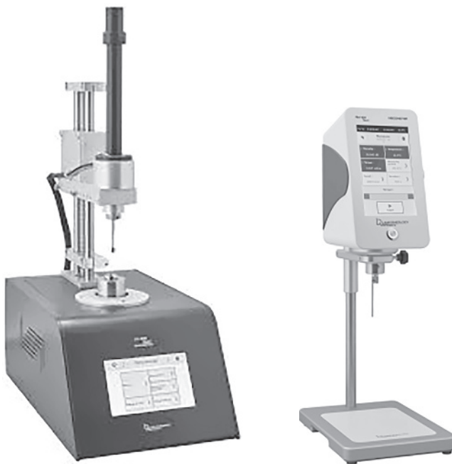
Figure 49.2 Rotating rheometers based on Couette principle. Source: With permission courtesy of M/s Lamy rheology.
