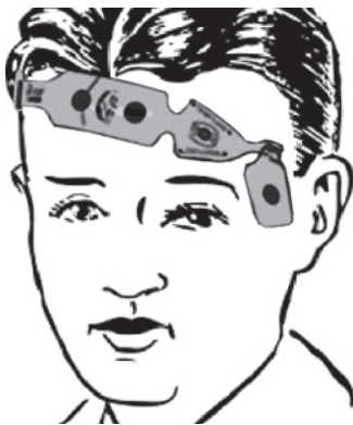
Figure 10.2 The location of sensor incorporating four electrodes for monitoring depth of anaesthesia.
