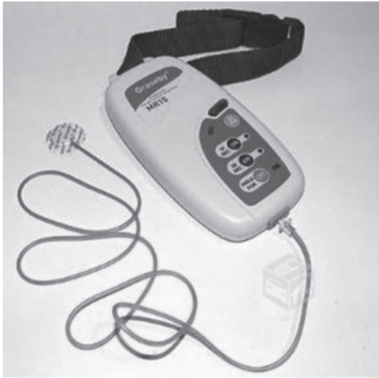
Figure 14.2 Apnoea monitor from M/s SIMS Graseby Ltd, United Kingdom, which consists of an encapsulated foam pad connected to a plastic tube. Expansion of the baby's abdomen with each breath produces changes in pressure, which are detected using a pressure transducer.
