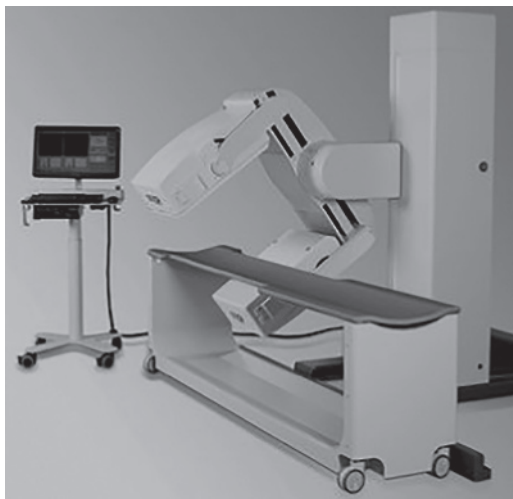
Figure 100.2 Dual camera SPECT scanner for performing a total body scan. The patient lies on a table that slides through the machine, while a pair of \gamma cameras rotate around the patient. Source: Reproduced with permission of M/s DDD-Diagnostic, A/s Denmark.
