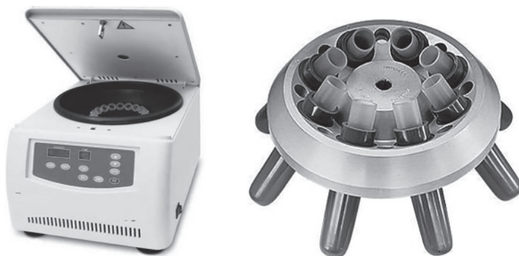
Figure 81.1 A typical laboratory centrifuge along with the details of the rotor.
