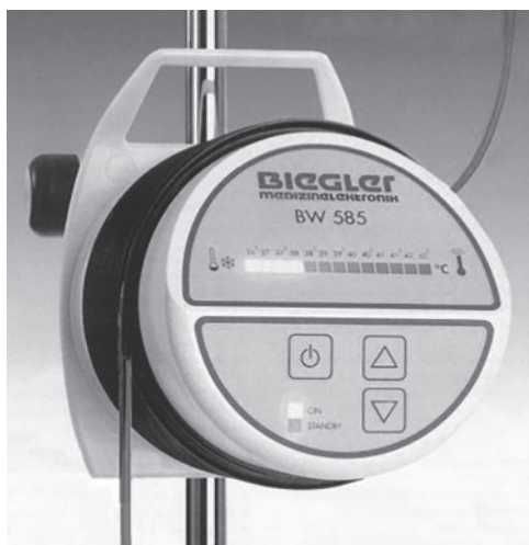
Figure 52.3 Typical blood warmer from M/s Biegler, Austria, with several loops to allow several infusions to be warmed at the same time.
