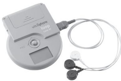
Figure 148.2 Cardiac loop recorder (from M/s Vitaphone GmbH, Germany) that uses ECG electrodes to acquire ECG signal.
