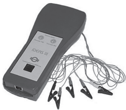
Figure 134.5 ENG signal acquisition instrument. The output can be given to a PC for data processing and display. Source: With permission of M/s DIFFRA S.A.
