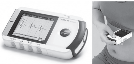
Figure 148.1 Cardiac event recorder from OMRON, which can pick up ECG signals by slightly pressing it on the abdomen.
