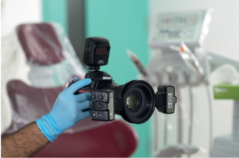
Figure 1.17 Bilateral twin flashes on a digital single lens reflex (dSLR) camera system.
