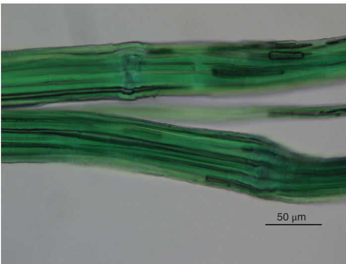
Figure 1.29 Longitudinal view of jute fibers using compound microscope – nodes are more visible than with the use of SEM.
