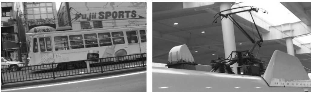
Figure 1.5 A conductively powered tram (left) and its pantograph (right), which is one of the oldest types of MPT.
