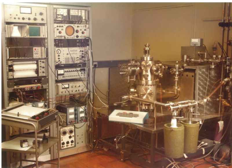
Figure 1.2 The system used at Mullards/Philips for modulated beam mass spectrometry measurements.
