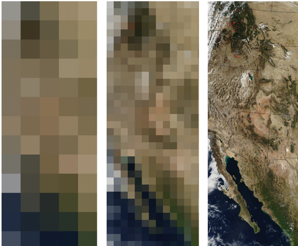
Figure 1.10 Satellite Images of the western coast of North America with different pixel sizes (grain). The general pattern can already be recognized in the image with intermediate grain. Source: Google Maps.
