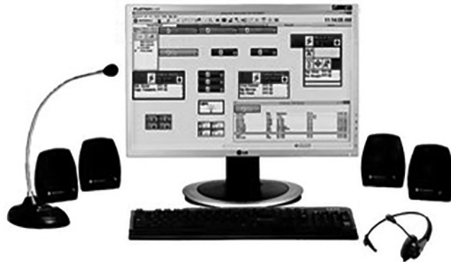
Figure 1.7. An example of a dispatch console [57].
