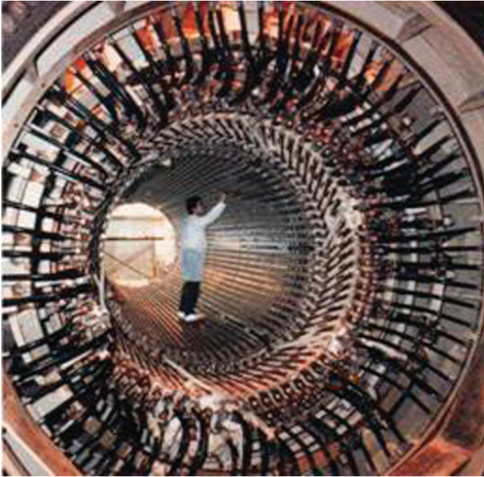
Fig. 1.34 Large modern generator stator with a rating of 2000 MVA or 1800 MW at 0.90 power factor. The weight of the stator is over 500 tons. The person standing in the bore gives perspective of the stator size.
