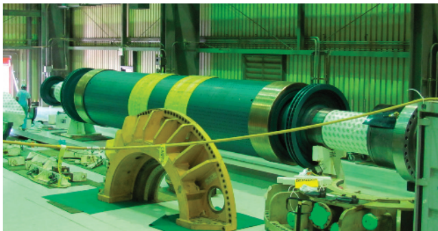
Fig. 1.35 Large 1600 MVA generator rotor. The weight of the rotor is approximately 250 tons. Note the person standing to the left of the photo who gives perspective as to the size of the rotor.
