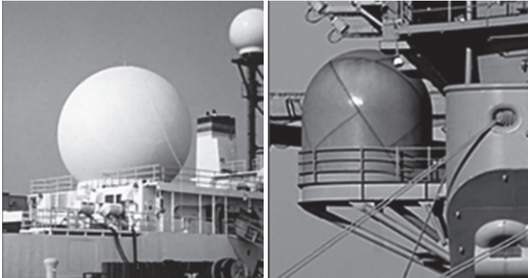
Figure 1.3 Typical radomes installed on ships.
