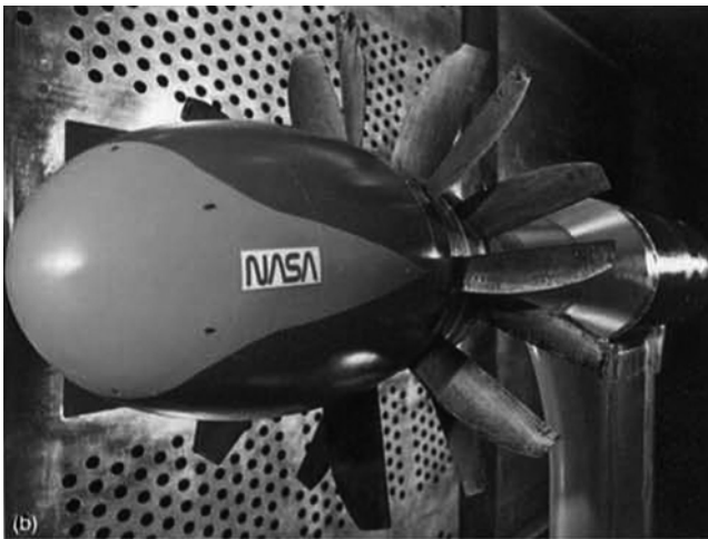
Figure 1.53 Unducted-Fan (UDF) counter-rotating model at NASA-Lewis (now Glenn) wind tunnel.
