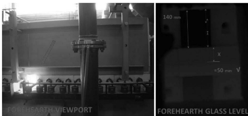
Figure 3. Forehearth Inspection Port and Forehearth Glass Level Estimate
