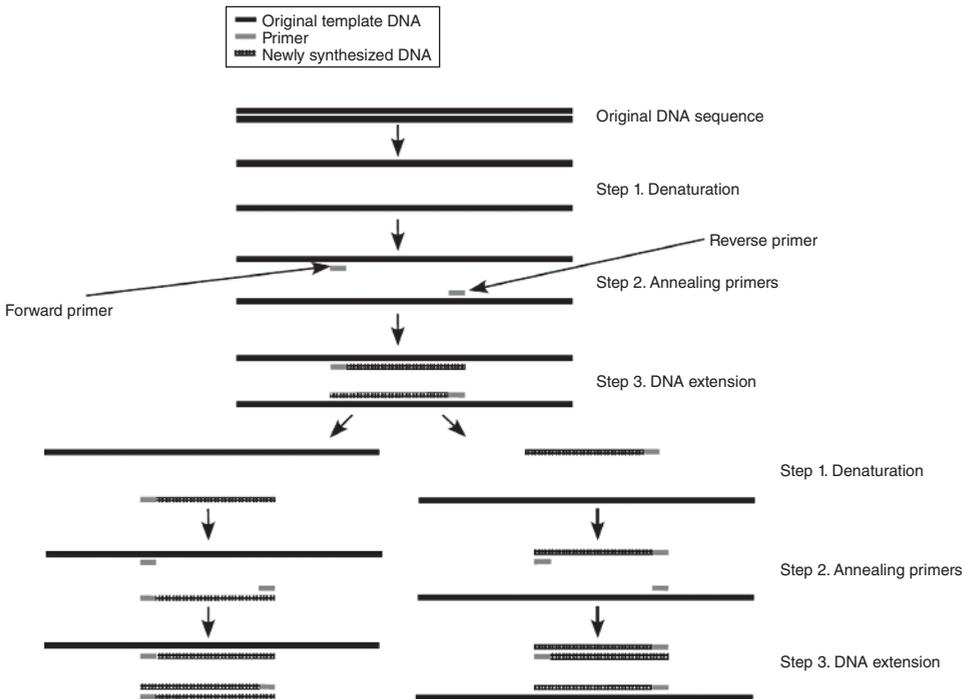
**Figure 1.13** The first two cycles in polymerase chain reaction (PCR). Solid black lines represent the original DNA template, short gray lines represent the primers, and hatched lines represent DNA fragments that have been newly synthesized.
