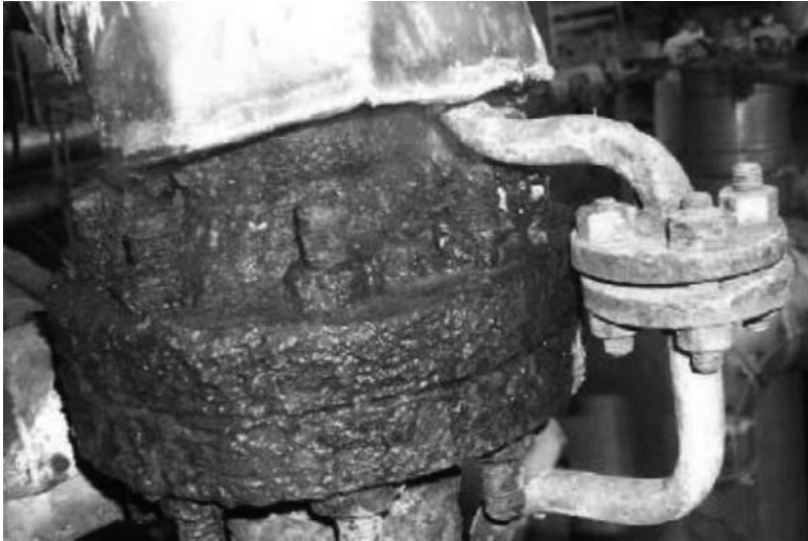
Figure 1.4-2. External Corrosion of a Pipe Due to Leakage of Steam Tracing (Sastry, 2015)
