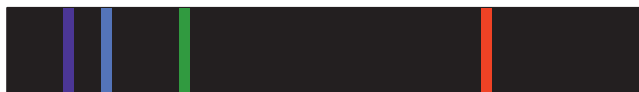
Figure 1.9 The emission spectrum of hydrogen that lies in the visible region of the electromagnetic spectrum, showing the four lines of the Balmer series.
