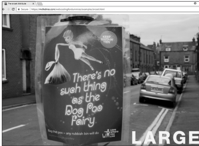
FIGURE 1-2: With the <img> tag's sizes and srcset attributes on the job, the browser serves up different versions of the image for different screen sizes.
