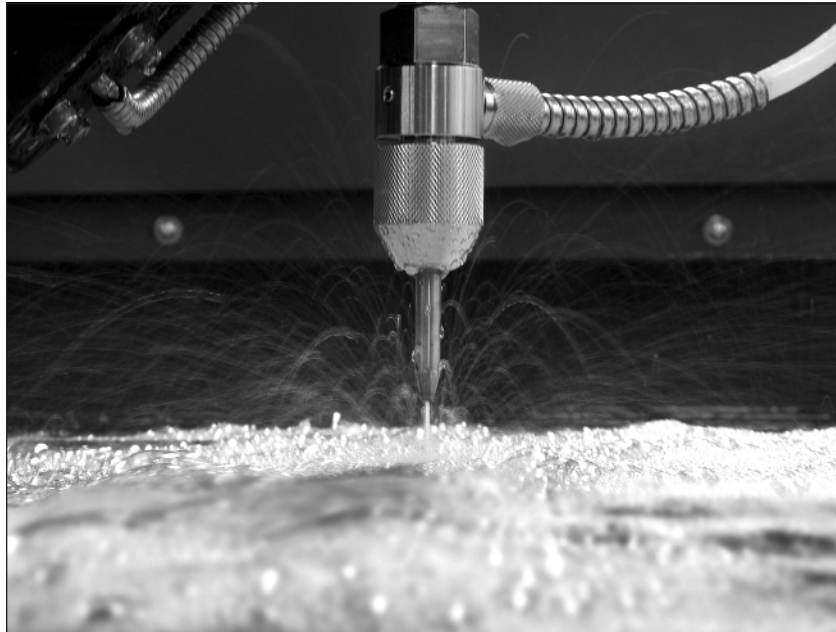
FIGURE 1-1: Abrasive waterjet machines can quickly and cleanly cut virtually any material in any thickness, from the hardest steel to the most friable stone.
