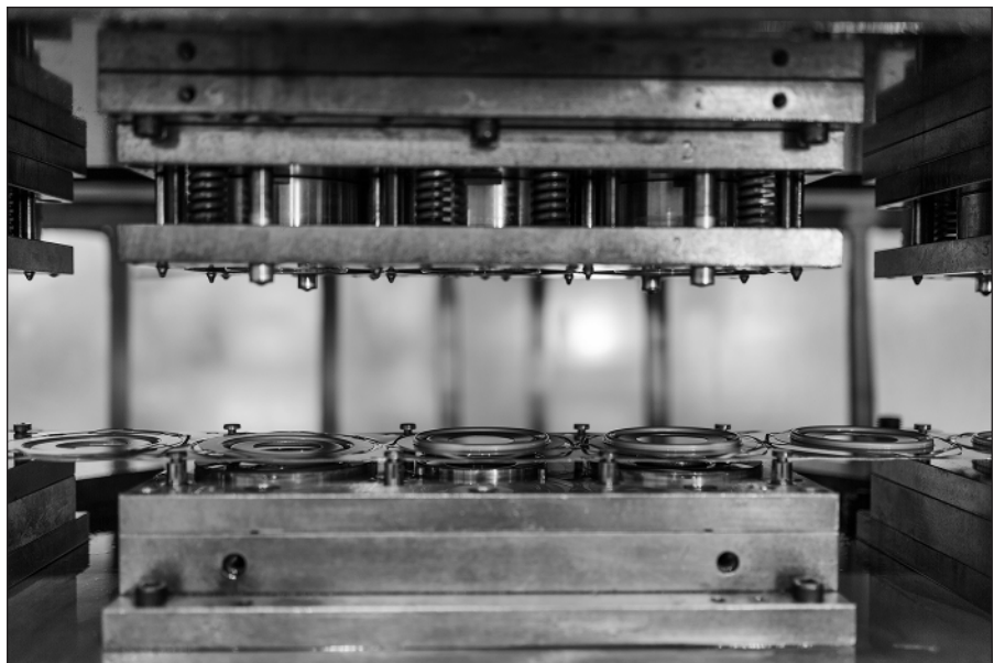
FIGURE 1-5: Progressive dies perform multiple successive stamping operations with each stroke of the ram.
