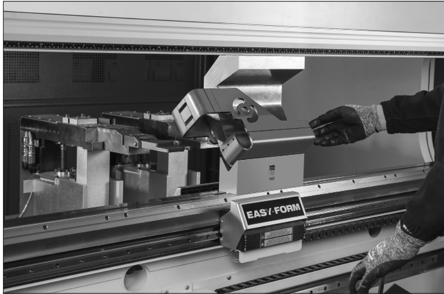
FIGURE 1-4: Bending complex parts like this is all in a day's work for a modern computer numerical control (CNC) press brake.
