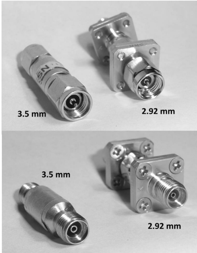
Figure 1.25 A 3.5 mm connector compared with 2.92 mm female (upper) and male (lower).
