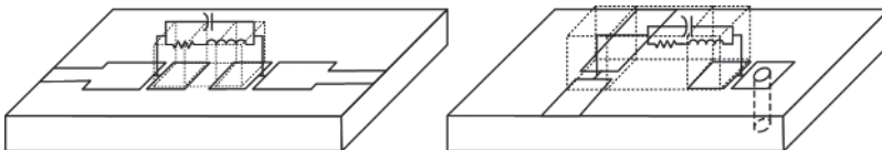
Figure 1.38 Models for a series resistor (left) and shunt resistor (right).
