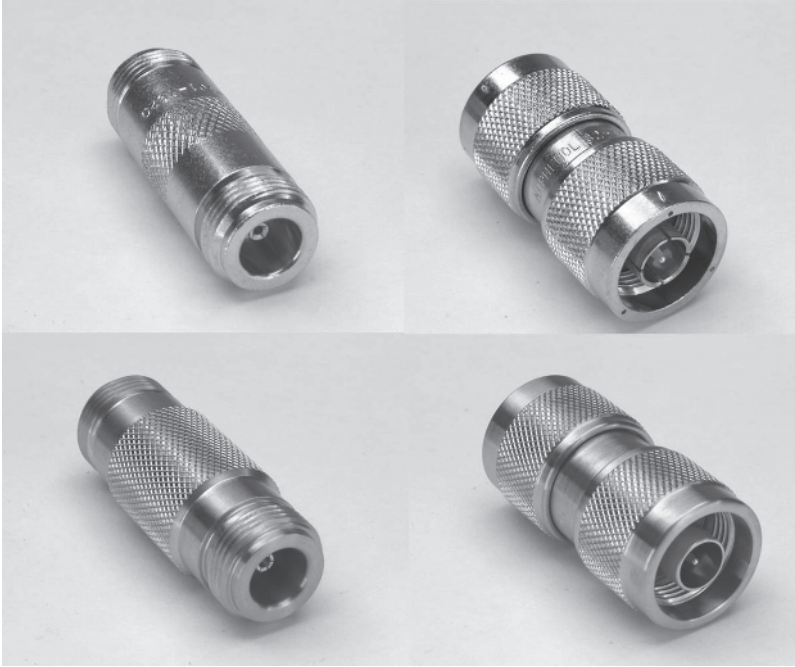
Figure 1.19 Examples of Type-N connectors: commercial (upper) and precision (lower).
