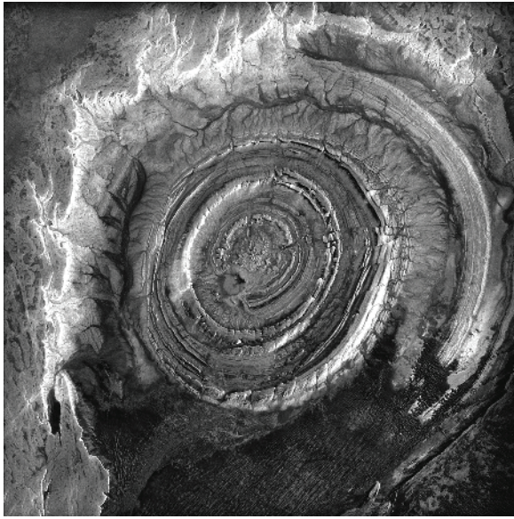
Figure 1.14 X-band synthetic aperture radar (SAR) image of the Richat geological structure in Mauretania collected by the Italian satellite COSMO-SkyMed 1 on 8 October 2007. The structure is about 60 km in width. COSMO-SkyMed (Constellation of small Satellites for Mediterranean basin Observation) plans to have five satellites in orbit eventually. The fourth was launched on November 2010. Source: COSMO-SkyMed Product ASI-Agenzia Spaziale Italiana – All Rights Reserved.
