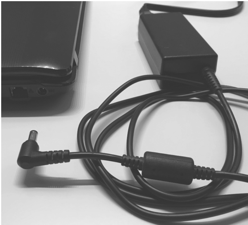
FIGURE 1.35 Laptop power supply
