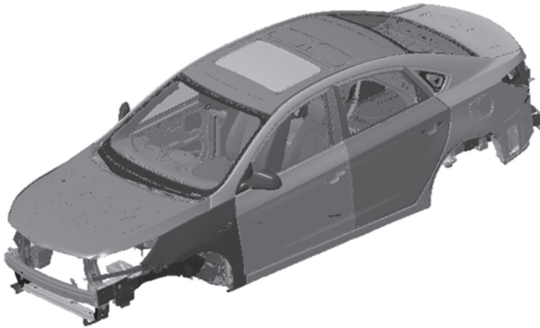
Figure 1.2 Structure of a trimmed body.
