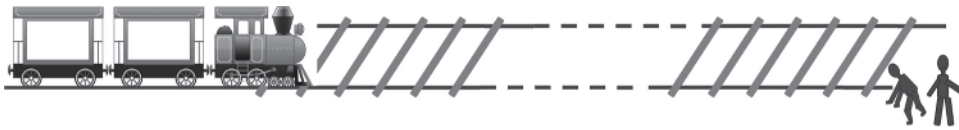
Figure 1.16 Transmission of structural-borne sound in rails.
