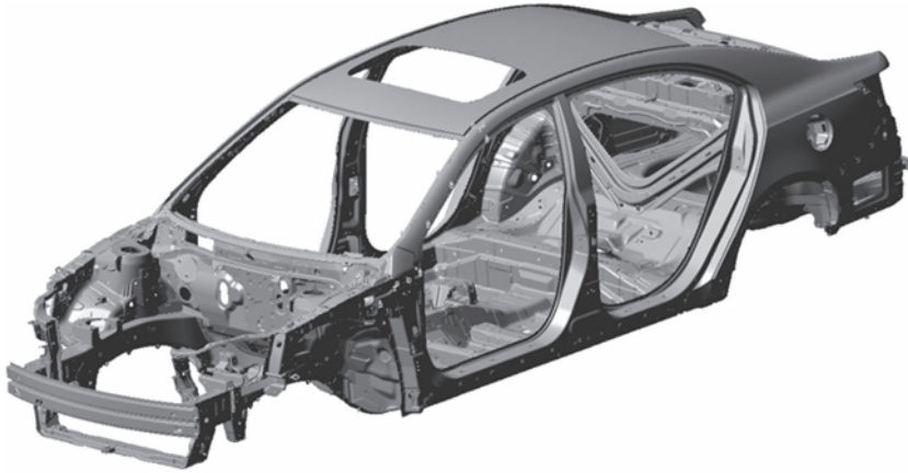
Figure 1.1 Structure of a united body.
