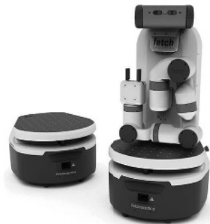
Figure 1.3: Example of a typical mobile robot, the Fetch series. The figure on the right shows the mobile robot base with an attached manipulator arm. (Photo courtesy of Fetch Robotics.)
