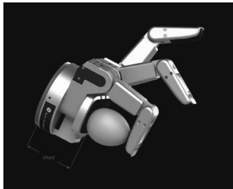
Figure 1.10: Anthropomorphic hand developed by Barrett Technologies. Such grippers allow for more dexterity and the ability to manipulate objects of various sizes and geometries. (Photo courtesy of Barrett Technologies.)
