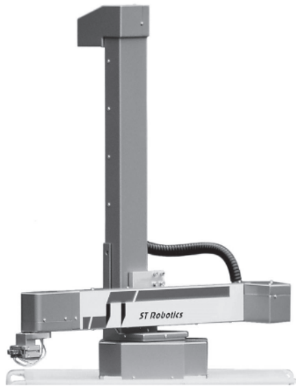
Figure 1.11 Cylindrical robot by ST Robotics. http://www.strobotics.com/index.htm .
