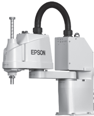
Figure 1.12 Epson Synthis™ T3 all-in-one SCARA robot. http://www.epsonrobots.com .
