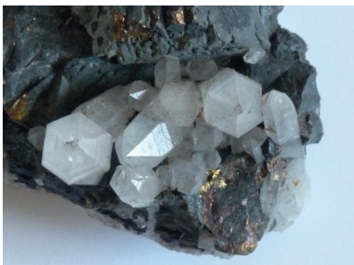
Figure 1.1 (a) Quartz ( \text{SiO}_2 ) crystals, showing hexagonal morphology; (b) pyrite ( \text{FeS}_2 , fool's gold) crystals showing cubic and octahedral morphology.
