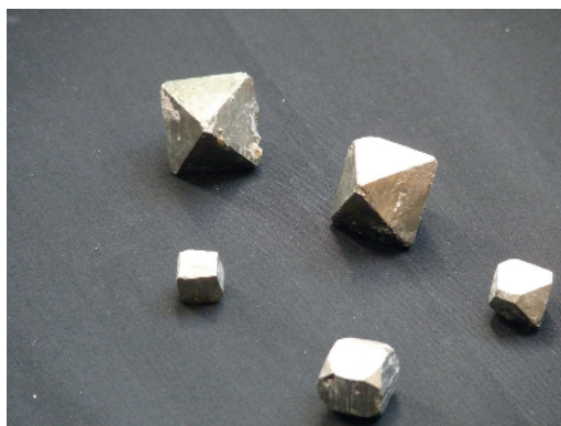
Figure 1.1 (a) Quartz ( \text{SiO}_2 ) crystals, showing hexagonal morphology; (b) pyrite ( \text{FeS}_2 , fool's gold) crystals showing cubic and octahedral morphology.
