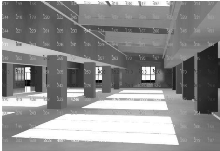
FIGURE 1.7 Daylighting overlay from Autodesk® 3ds Max®
