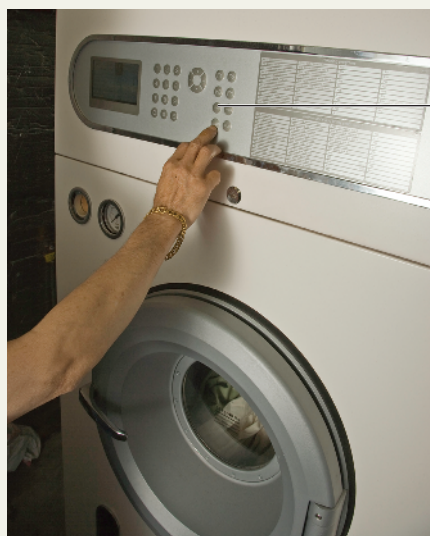
Controls for regulating flow of dry-cleaning liquids
