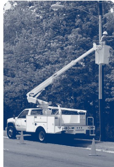
(b) Telescopic aerial device. (Used with permission of Altec Industries.)
