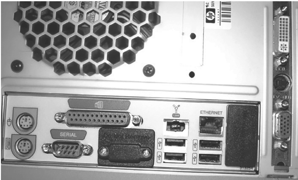
FIGURE 1.3 Common ports (PS/2 keyboard and mouse ports, serial port, parallel port, 1394 port, several USB port, Ethernet port, DVI-I port, and VGA port)
