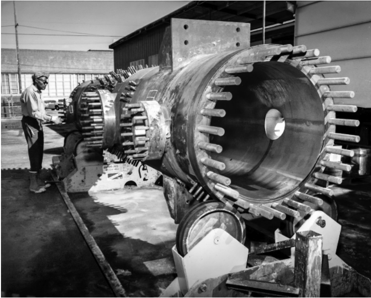
Figure 1.2 A vessel fabricated with a heavy wall to minimize cost (Source: Los Alamos National Laboratory)
