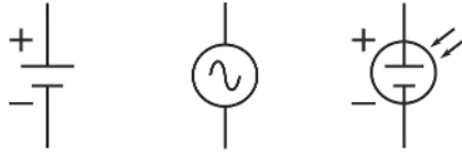
FIGURE 1-9: Circuit symbols for a battery (left), AC power source (center), and photovoltaic cell (right).
