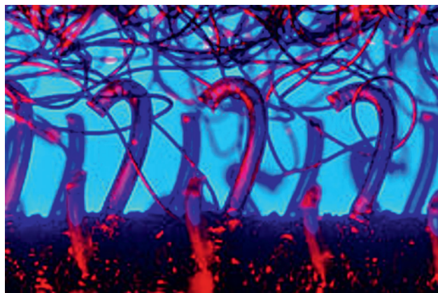
Figure 1.4 The structure of hook and loop fasteners.
